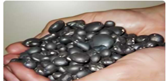
Iron Nuggets manufactured through ITmk3
